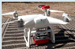
Above: 2016 DJI Phantom 4 drone with RedEdge MicaSense camera
